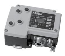
The IDENT Control Interface is the backbone of the entire RFID system. It connects directly to your PC/PLC of choice and manages all communications to and from the 4 read heads. Read heads are configured on power up, and parameters, like multiplex mode and tag type, are set automatically.
